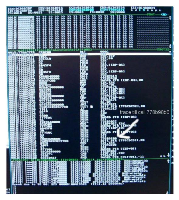
Now we are in the RTLTraceDatabaseEnumerate API which we pass best buy using the F10 key in softice till the call 778b98b0 and step into this one buy using the 't' command.
