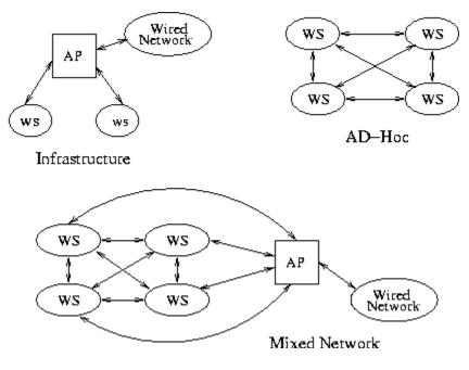
Fig2.1: Types of WLAN
