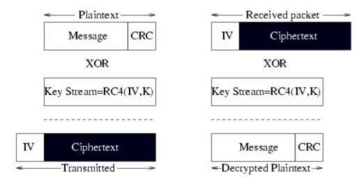
Fig 3.4: Encryption & Decryption on WEP
